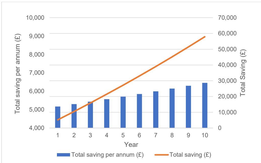
Figure 22: ROI for reflective roof on an office building in London (with a low insulation roof) (Arup)
